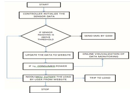
Figure 5.1 Flow Graph of Working
