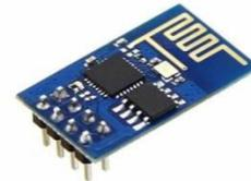
**Figure 8.1 ESP8266 Wi-Fi Module**
