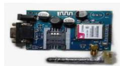
**Figure 7.1 GSM Module**
